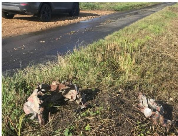
Further examination revealed it to be aviation grade lightweight aluminium and the pieces appeared to have experienced a high-speed impact. Additionally, and importantly, the items were painted red, albeit very faded. The conclusion that the items came from the stricken USAF aircraft was made by Ian Brown, the curator of the RAF Sculthorpe Heritage Centre.
